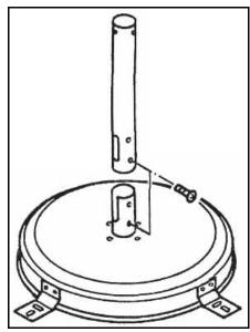
Connect all center post sections together. Secure with screws.
