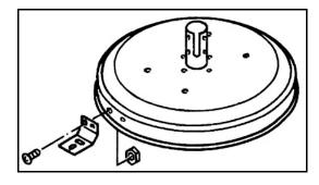
Place base post on the bottom of the base in upward position.
