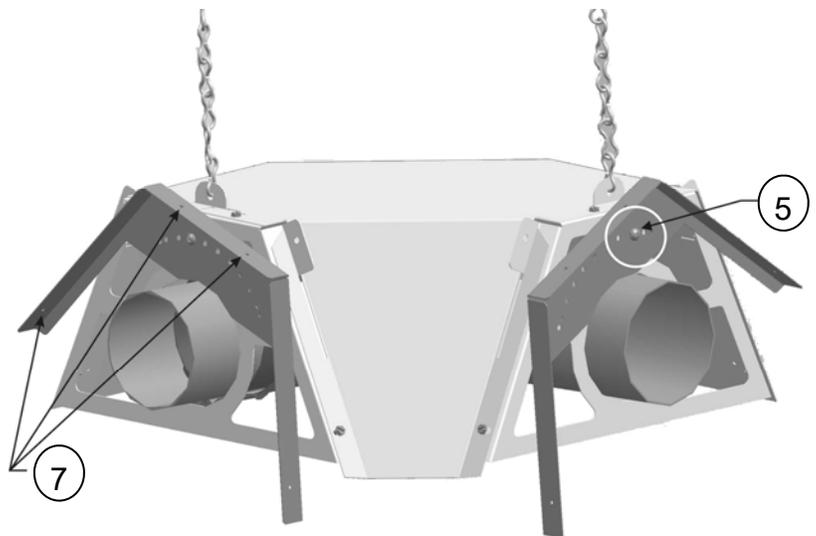
4. Align one of the holes in the angle adapter with the hole at top center of the elbow/tube hanger
