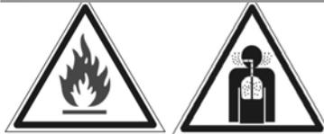
Inadequate venting of a heater may result in asphyxiation, carbon monoxide poisoning, injury or death. This heater may be directly or indirectly vented from the space. Venting must be in accordance with all local, state, provincial, and national codes (ANSI Z223.1/NFPA 54 in USA; B149.1 in Canada) and as indicated in this manual. **Refer to Sections 11 & 12**
