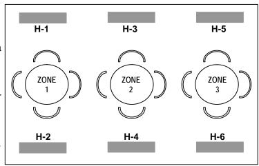
Similarly, set receivers in heaters **H-3** & **H-4** to "2" and **H-5** & **H-6** to "3". Both Zone 2 heaters turn On/Off with button set "2" and both heaters in Zone 3 with button set "3".
